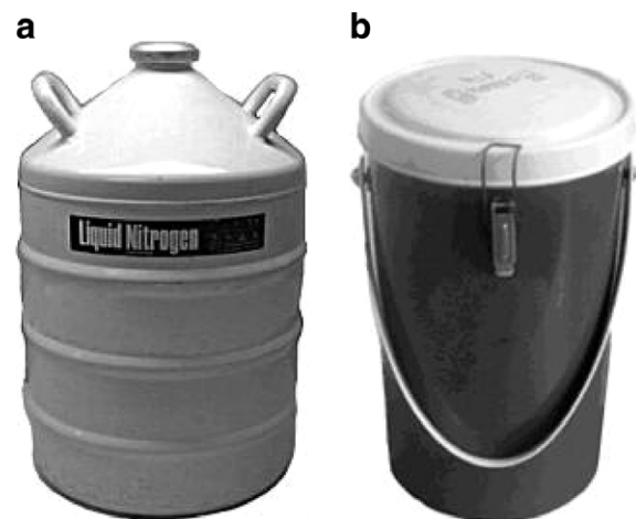
Fig. 3 – (a) A picture of a dewar, characterised by a narrow mouth, is depicted which is a holding tank for liquid nitrogen. From that device, liquid nitrogen is poured into some other device, e.g. a transportable refrigerator shown in (b). The shaking flask (Fig. 6e) is precooled in such a refrigerator for about 5 min and then transferred immediately to the shaking device (holder) (Fig. 6b) of the Mikro-Dismembrator S (Fig. 6a).
